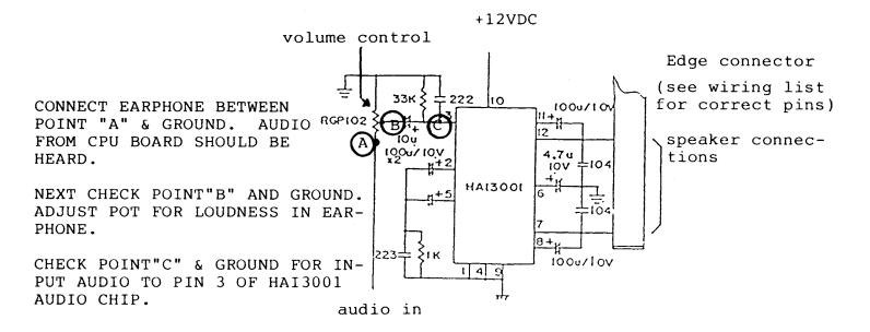
Also make sure Ground from  $+5 \, \text{VDC}$  and Ground from  $+12 \, \text{VDC}$  ARE TIED TOGETHER. IF GROUNDS ARE FLOATING, you could have audio problems.
